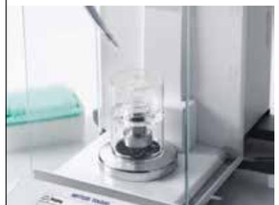
For routine pipette testing, an evaporation trap significantly reduces moisture loss of the test liquid and can be mounted on your balance in seconds.
