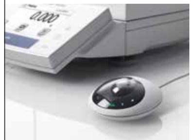
ErgoSens enables you to perform selected balance operations with the wave of a hand e.g. zero, tare, print. Processes are simplified and cross contamination is avoided.
