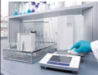
The full weighing chamber, including SmartGrid and the drip tray underneath, dismantle in seconds and all parts go in the dishwasher.
