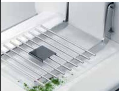
SmartGrid minimizes the effects of air currents to substantially reduce stabilization times. Spilled substances fall through the grid and don't influence weighing results.
