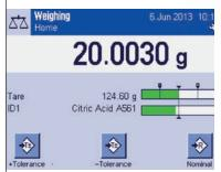
The color-guided SmartTrac<sup>™</sup> function makes it easy to dose to your target weight and stay within tolerances. Using the appropriate ErgoClip enables you to dose directly into your container in one easy step.
