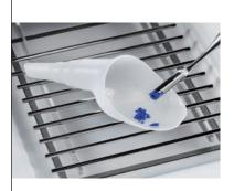
The single use SmartPrep<sup>™</sup> weighing funnel is made from antistatic material and is intended for the simple and safe weighingin of powders. The unique design allows easy-access dosing and enables powders to be effectively rinsed off into your desired flask, thus minimizing sample loss.
