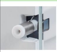
The new compact antistatic kit can be used to gently generate charged ions and hence eliminate electrostatic charge without causing turbulence in the weighing chamber. The steady stream of ions prevents cross-contamination of samples and removes the threat to users when handling toxic substances.
