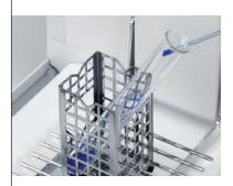
The ErgoClip<sup>™</sup> basket acts as a Faraday cage to shield the balance from any electrostatic charge which could be present on glass and plastic tubes. Weighing samples in tubes is therefore more safe and reliable.
