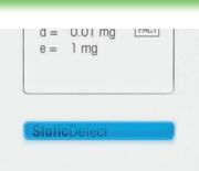
Our StaticDetect<sup>™</sup> technology detects electrostatic charge on the sample and/or its container. The weighing error is measured and a warning is given if the user-defined limit is exceeded. Antistatic measures can then be employed.
