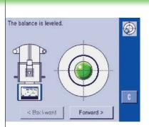
The new LevelGuide<sup>™</sup> provides you with a warning when the balance is not level. Full instructions and a graphical bubble are shown on the touchscreen so you can level your balance in seconds.
