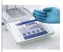
The enhanced touchscreen user interface offers tireless, intuitive balance operation. SmartSens<sup>™</sup> sensors allow you to operate your balance with the wave of a hand, making weighing tasks easier and avoiding cross-contamination issues (e.g. opening/ closing draft shield door).
