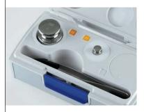
CarePacs<sup>®</sup> contain just what you need to test your balances in accordance with USP 41 – two test weights corresponding to 5% and 100% of the capacity of your balance. Tweezers, gloves and other accessories are included for professional weight handling.
