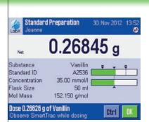
LabX provides step-by-step user guidance on the balance touchscreen so you can be sure your SOP is followed precisely. Centralized instrument management means all your balances automatically display the same SOP instructions to guarantee consistency in your lab.
