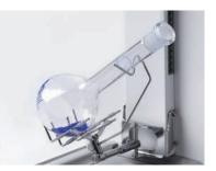
One step dosing directly into the tare container eliminates transfer errors and saves money by minimizing sample loss. Even unusual shaped containers are held securely in place. In combination with the MinWeigh Door<sup>™</sup> accessory, ErgoClips help you achieve the lowest possible minimum weight.
