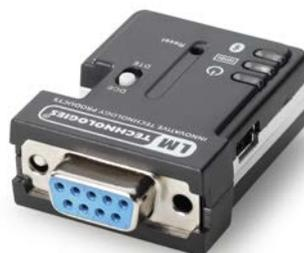
Simply plug in the BT adapter where there is no built-in BT interface to wirelessly send data between your balance and a PC, tablet or printer.
