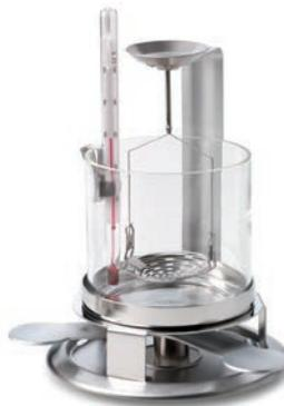
Density determination of solid and liquid samples is easy with this kit for analytical and precision balances.
