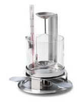
Density determination of solid and liquid samples is easy with this kit for analytical and precision balances.
