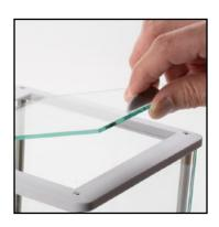
Periodic cleaning made easy helps to avoid sample contamination and extends product life. In addition, a standard in-use cover provides added protection against accidental spillage and helps minimize the chance of damage to the display and keypad.
