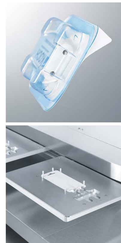
Below: Pallet transport system at ergonomic height for blister loading
