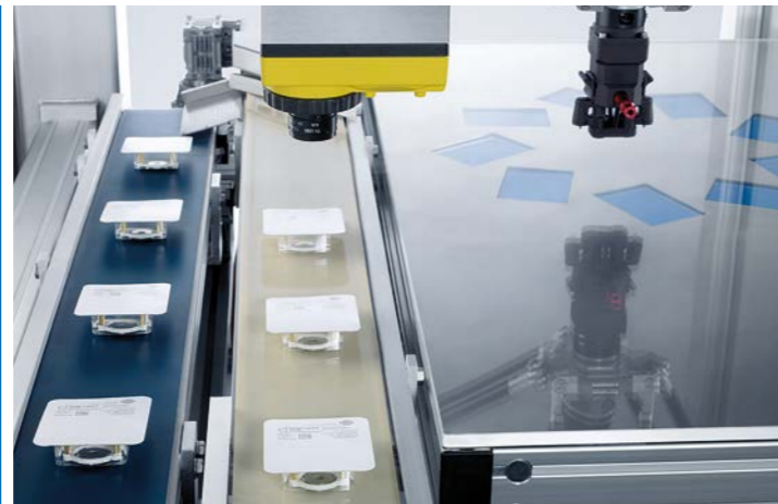
Exemplary marking and inspection system that prints and subsequently verifies variable product data
