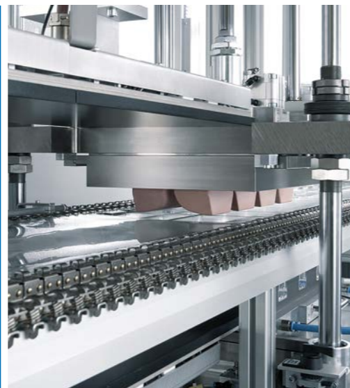
Chain transport with forming station
