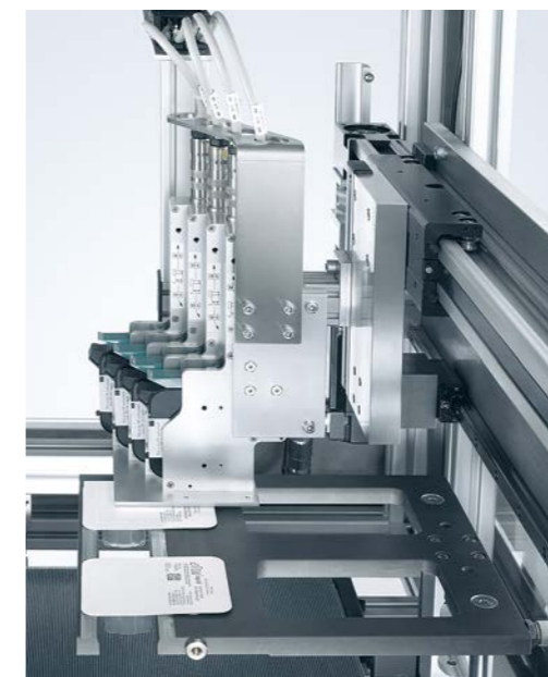
Thermal inkjet printing system with four print heads for the marking of blister cards
