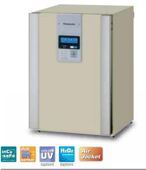
CO<sup>2</sup> level: **0** — **20%** O<sup>2</sup> level: **1** – **18%**, **22–80%** Temperature: Ambient temperature **+5°C** — **50°C** Interior volume: **162 L (5.7 cu.ft.)**
