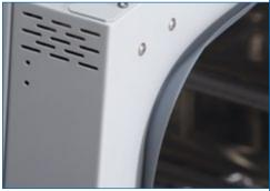
The gasket flange on the inner door faces towards the laboratory environment keeping unwanted growth isolated from the growth chamber. The gasket may be removed and autoclaved separately if so desired.
