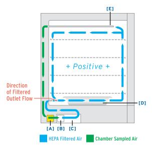
[A] HEPA Filter [B] Air Pump [C] Sensor Bay [D] Water Pan [E] Air Inlet Tube
