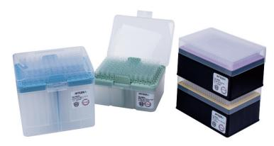
GripTips are packaged in two different tip racks dependent on the pipette tip volume. Larger volume GripTips, 300  $\mu$ l and 1250  $\mu$ l, are packaged in racks of 96 tips. Smaller volume GripTips, 12.5  $\mu$ l and 125  $\mu$ l, are packaged in space efficient racks of 384 tips. These XYZ racks contain four times as many tips and are molded from an anti-static material to prevent static build up.
