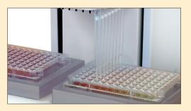
Performing serial dilutions and mixing of entire plates is easily accomplished. The number of mixing cycles and mixing speed can be exactly defined.
